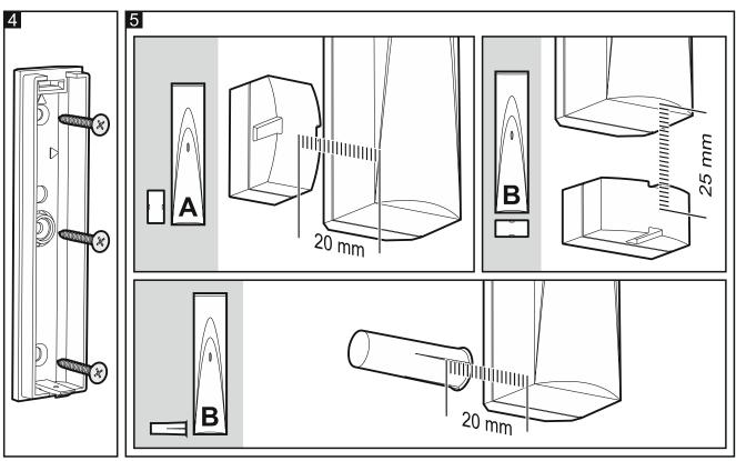
8. Secure the magnet, taking into account the maximum permissible distance from the reed switch (Fig. 5). The distance shown applies to the magnet located at the reed switch height. Location of the reed switches in the enclosure is shown in Fig. 3.
