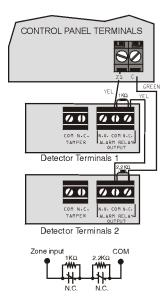
N.C. Contacts, with EOL, with Tamper and Wire Fault Recognition (UL/cUL)
