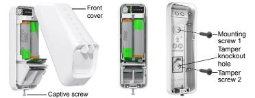
Figure 1 – Removing the Front Cover
